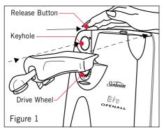
The Cutting Assembly fits into the keyhole opening at the top of the Open All<sup>™</sup> can opener, above the Drive Wheel. Slide the Release Button to the right as the Cutting Assembly is inserted, it will "click" into position, with the release button returning to its original position.
